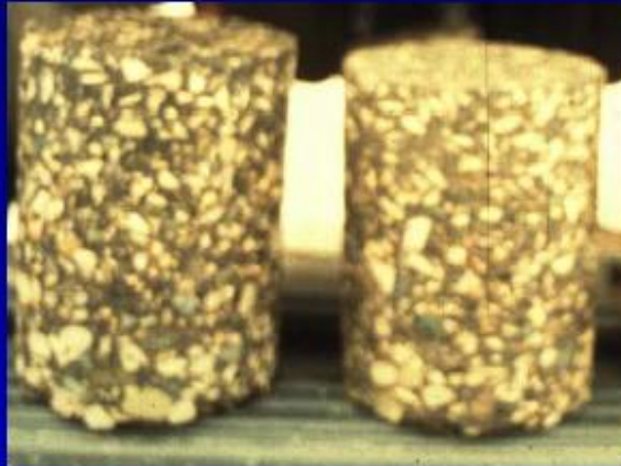
TYPICAL CIR STABILIZED BASE CORES
